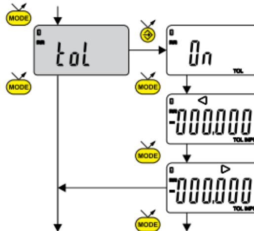
.....Input the lower tolerance limit
