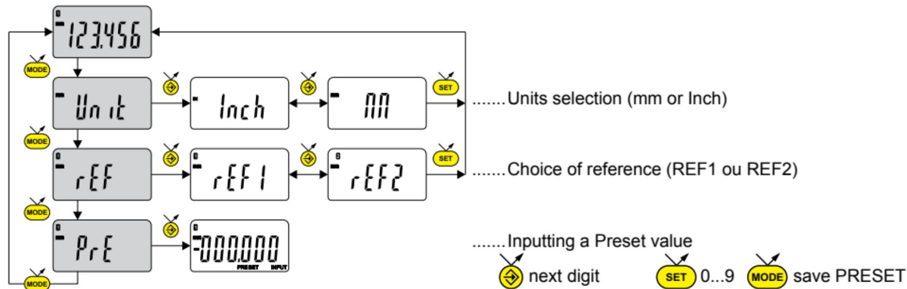
**Note:** It is possible to assign a different preset value to each of the 2 References. Similarly, different tolerance limits can be assigned to References 1 and 2.
