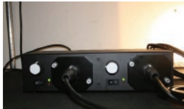
Metal Halide Light Source for Ultra-Precise Wafer Positioning During E-Beam Metrology circa 2005
