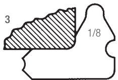
Fig 3. Checking convex (external) radius with 90° arc. Also checks if sides are tangent to radius and 90° to each other.
