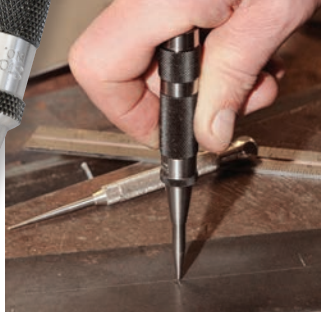
Rugged automatic center punch with adjustable stroke
