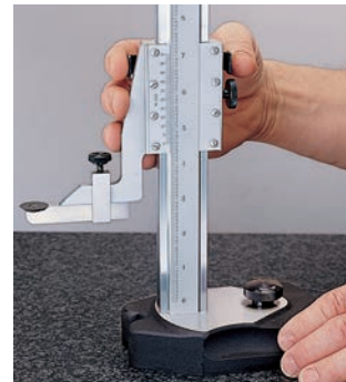
Quick-adjusting screw release allows rapid slide movement to desired area, then precisely position with the fine adjustment knob
