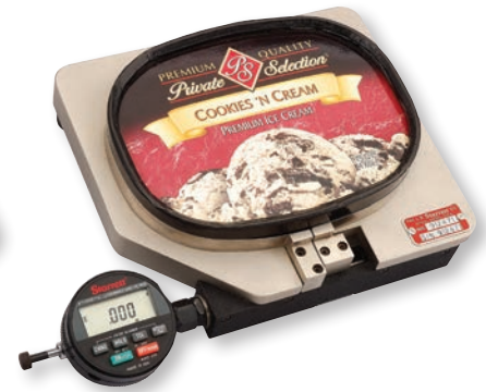
Top of 1/2-gallon container in measuring position
