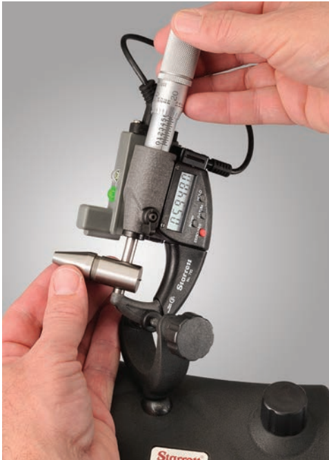
795XFL-1 with a DataSure End Node
