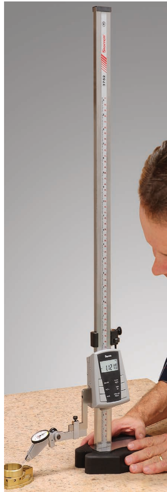
Height gage with PT99454 indicator holder with 790AZ test indicator
