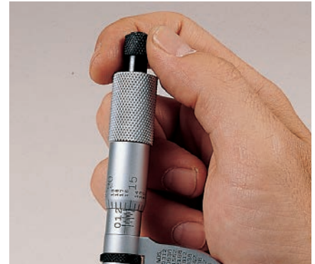
Ratchet stop/speeder for consistent measurements and to speed opening or closing of tool.
