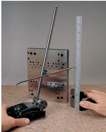
Transferring measurements with a Starrett Surface Gage used in conjunction with rule and rule holder
