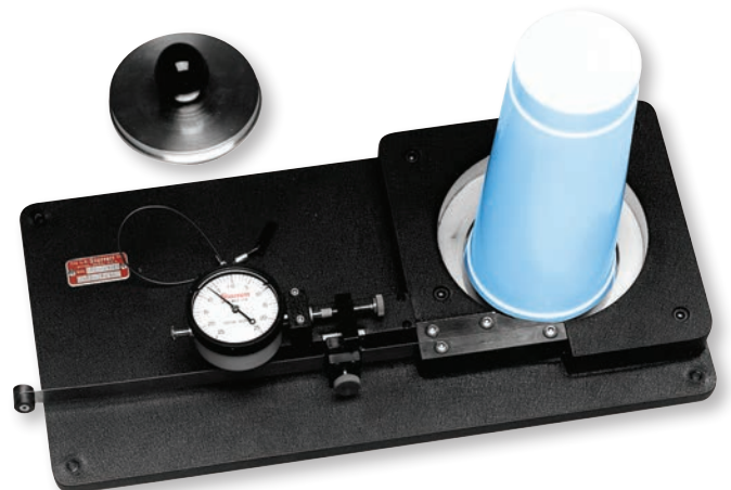
Top of 1/2-gallon container in measuring position
