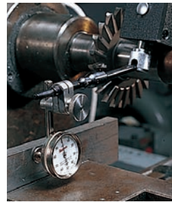
657A with 196B1 Universal Dial Indicator setting up workpiece on milling machine.
