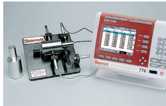
The 776 accepts multiple gage inputs simultaneously – invaluable for applications such as this Starrett special gage fixture
