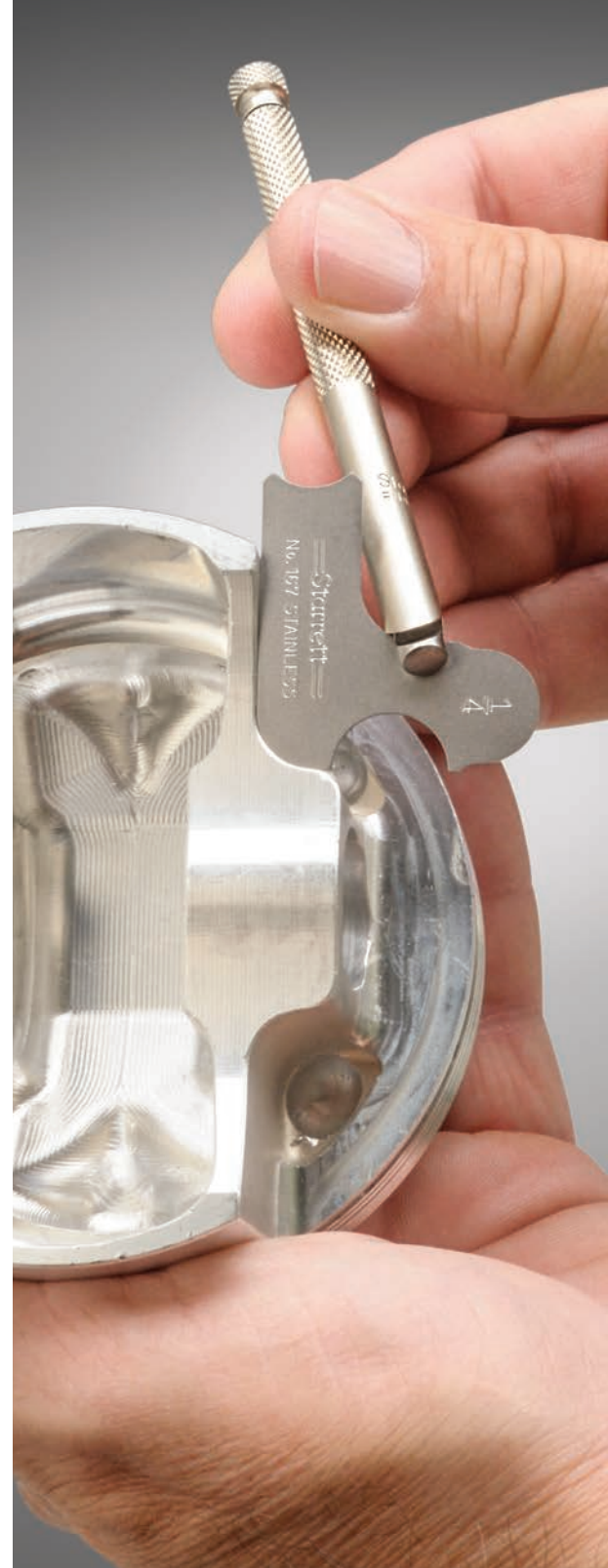
Gaging radii using gage with holder
