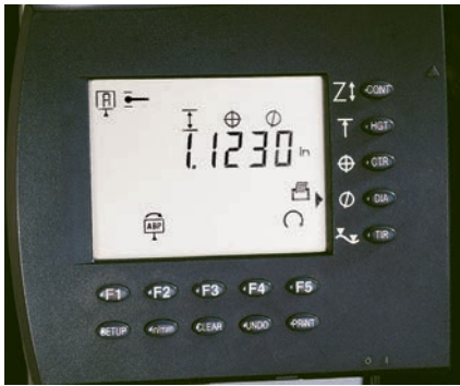
Large, easy-to-view /understand display shows the diameter of a hole or boss
