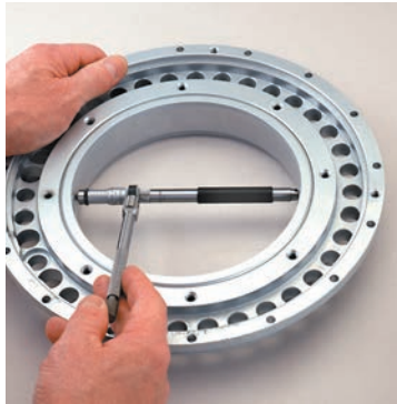
Rods attachable as shown to either one or both ends of the head ensures the best balance, feel, and ease of reading.
