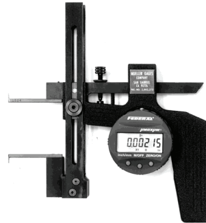
Model 1904 with Analog/Digital Indicator
