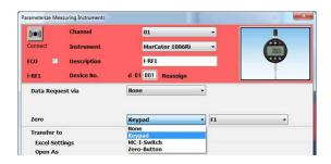
Here the type of action can be selected in which the RF device gives the command for zero setting. Whilst "Keypad" and "MC-I Switch" function identically to that of Data Request it is also possible to create an additional button on the user window which is clicked with the mouse.
