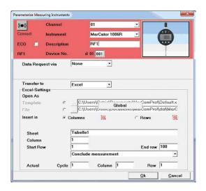
12. In the Checkbox "ECO" you can activate the energy saving mode for the wireless data transmission, thus reducing energy consumption of the integrated wireless wire measuring instrument up to 30 %.
