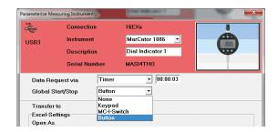
Additionally, a pull-down menu for starting and stopping the timer is available. You can select whether the timer is to be also started and stopped via a function key (e.g. F1), MC-I switch (e.g. foot switch) or global via the timer button in the status window. In this way several timers for various measuring instruments can be simultaneously started and stopped.
