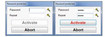
In order to revoke the password protection, enter the password and then press Abort. To reactivate a password simply enter any desired password, repeat the process a second time, subsequently activate the password protection with the Activate icon.
