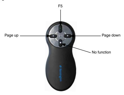
The Remote Control (4102221) no external driver is required. Once a USB receiver has be connected Windows own driver will be installed. After the this driver has be installed you can press a button on the remote control which simulates a keyboard command, see above illustration. With MarCom these keyboard commands can be assigned functions.
