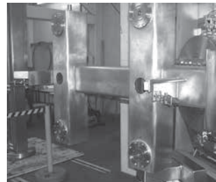
Jergens Zero Point clamping systems are made exclusively of rust-free materials and so are ideally suited for use in the food-service area as well as in the pharmaceutical and chemical industry.
