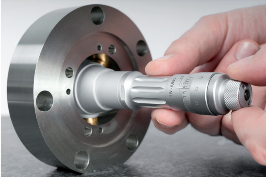
Bore measurement with a BROWN & SHARPE INTRIMIK inside micrometer
