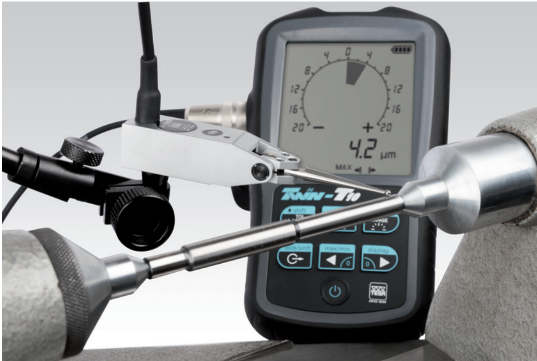
Run-out measurement with TWIN-T10 and GT 31 lever probe
