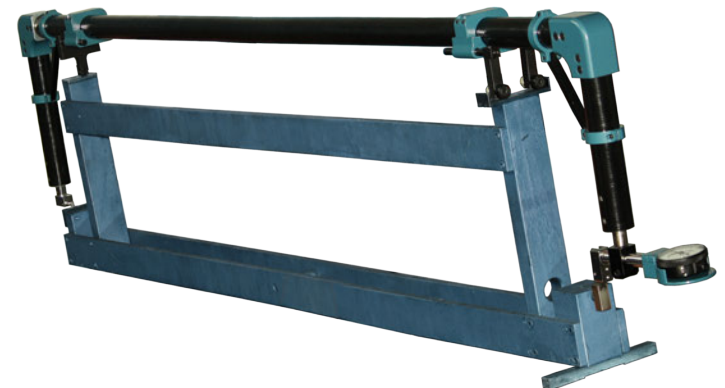
Special carbon fiber frame gage with master
