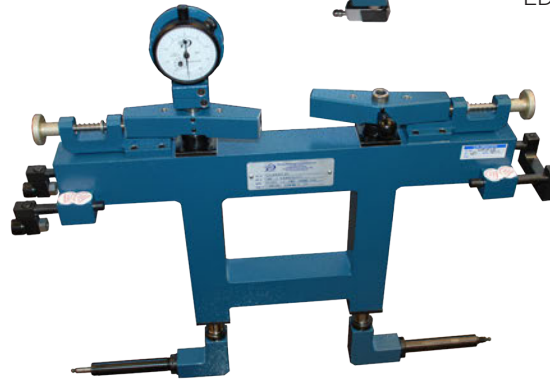
LD - Swing gage, where the heads rotate inward for long retraction
