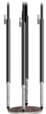
6 mm probes checking the thickness of a coin
