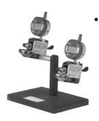
By mounting multiple gaging frames on the same base and using functional elements on one frame and using pitch diameter elements on the other frame differential gaging can be made easy by making quick machine adjustments before bad product is produced. Available with digital read out and RS232 outputs.
