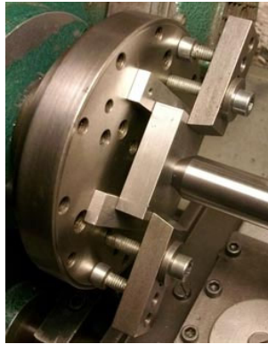
Centering a workpiece in a machine tool
