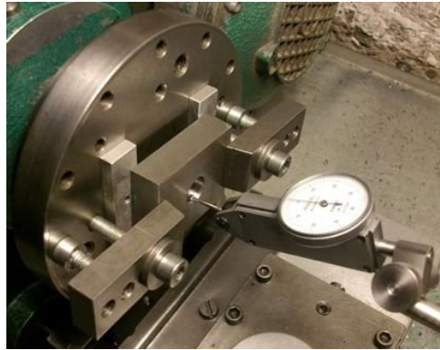
Centering a workpiece in a machine tool
