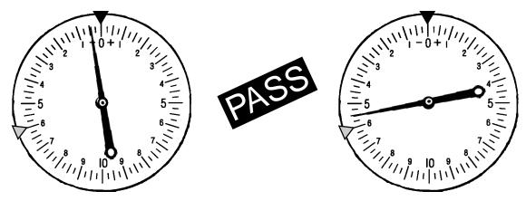
The quality of the thread form is poor. However, it is still within acceptable Pitch diameter tolerance limits. This product passes Systems 21 and 22. May not pass System 23.
