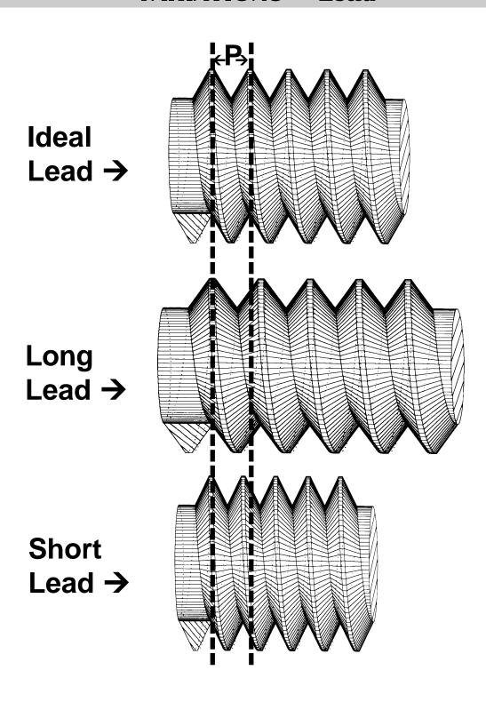
Lead is the axial advance per unit rotation for a given pitch distance.
