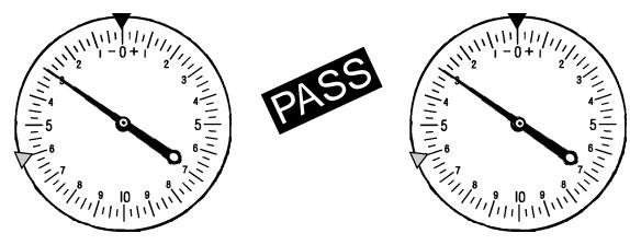
The quality of the thread form is ideal. The thread size is positioned at the mean of the Pitch diameter tolerance. This product passes Systems 21, 22 and 23.
