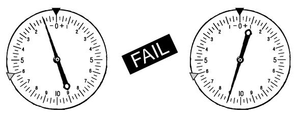
The quality of the thread form is poor. Pitch diameter size has exceeded minimum material limit. This product fails Systems 22 and 23, but may pass System 21.
