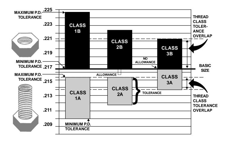
Classes of threads are differentiated by the amount of tolerance and allowance specified. Indicating gaging is typically mastered at maximum material condition. This is the minimum Pitch diameter tolerance limit for I.D. threads and the maximum Pitch diameters tolerance limit for O.D. threads.
