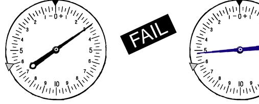
The quality of the thread form is poor. Functional diameter size has exceeded the maximum material limit. This product may not assemble. Product fails Systems 21, 22 and 23.
