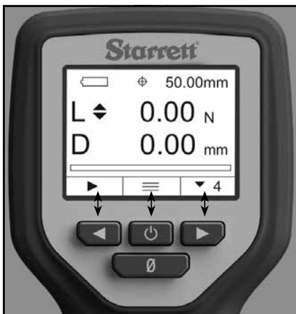
Shown: Keypad mapping with display in NORMAL format
