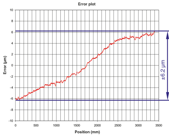
Example accuracy test result of 3400 mm length of RTLC scale
