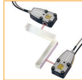
RLD10 double pass interferometer
