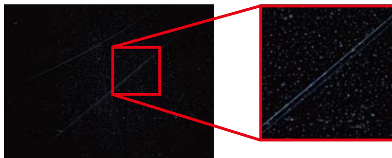
Dark-field: Allows highlighted observation of microscopic abnormalities such as flaws and contamination by using diffused light.
