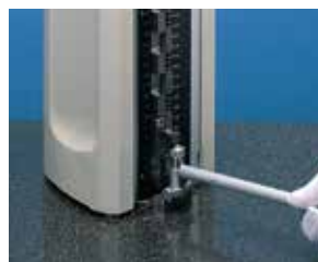
Using height master to set bore gage
