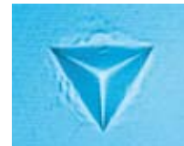
Indentation by triangular pyramid indenter
