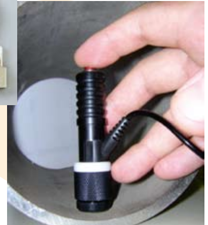
● Hardness testing of internal walls of pipes and tight spaces
