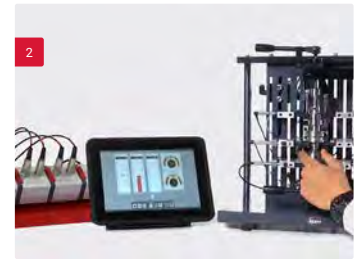
Shaft measurement with inductive modules
