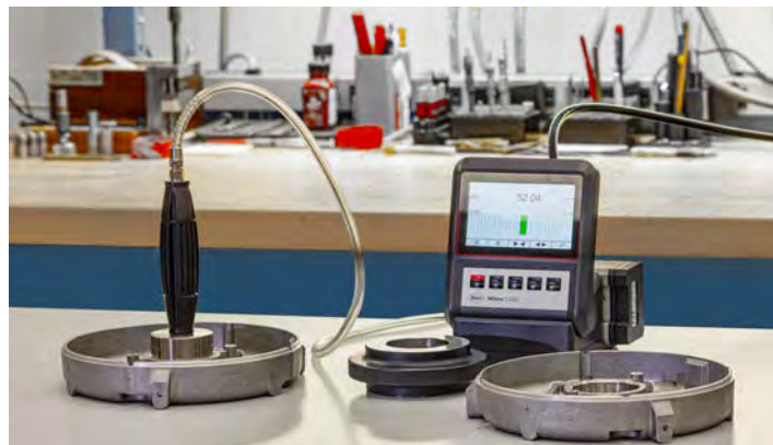
Stand alone air gaging for bore diameter
