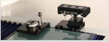
Master ball (option) Calibration ring (option) Used for offset calibration of the image and the touch probe.
