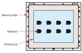
Continuous measurement of multiple workpieces
