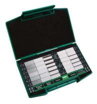
For checking, identifying and specifying the roughness by symbol
