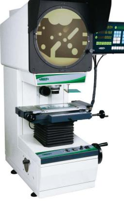
overlay chart (protractor with 1° graduation, radius with 1mm/.039" increment)
