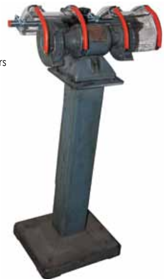
Shown Above: Pedestal Mount Grinder Guard Deluxe with adjustable mounting hardware.
