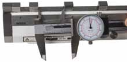
Checking the accuracy of Calipers by internal jaw
