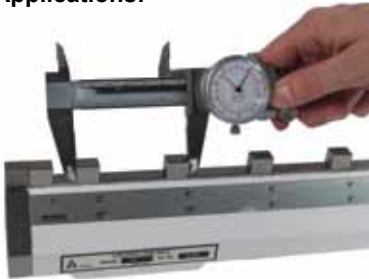
Checking the accuracy of Dial Calipers by external jaw
