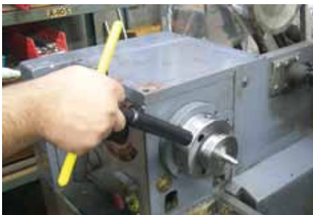
Adjusting the chuck using a spring-load chuck wrench
