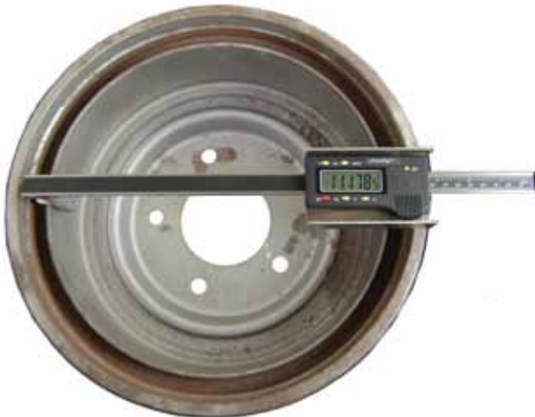
Shown Above: Internal Drum Diameter Measurement
