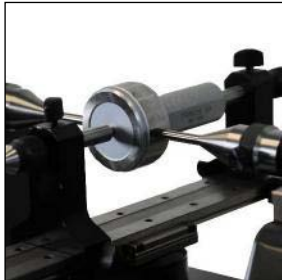
Checking of plug gages and pin gages, Max. \phi 100mm/4", length 280mm/11" (TULM6/L0.5, LABC15)
