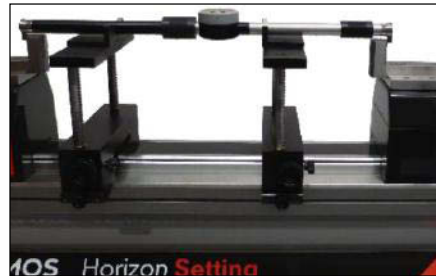
Setting of 2 point internal and external comparative measuring equipment (TEL5, TELMA7, TELMN7.2)
