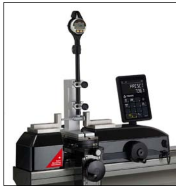
Setting of 2 point bore gages with holder (TA-SU-313, TA-SU-318, TEL5)
