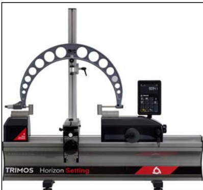
Checking of external micrometer held on a support (TA-SU-309, TA-SU-309, TEL5)
