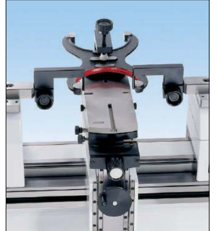
Checking of snap gages with range from 0.473 to 6"/12 to 150mm using table (54-197-011-0), snap gage holder (54-197-014-0) & L-probes (54-197-162-0)
