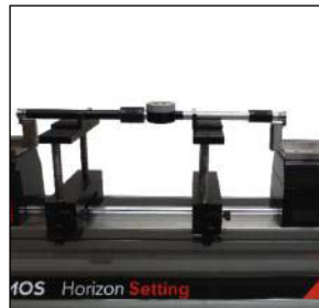
Setting of 2 point internal and external comparative measuring equipment (TEL5, TELMA7, TELMN7.2)
