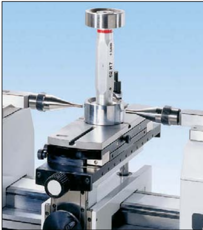
Checking of plug gages and threaded plug gages from dia. 1.18" to 10"/30 to 250mm using table (54-197-011-0), clamps (54-197-142-0), small Ø anvils (54-190-806-0) & thread wires (54-197-007-0)
