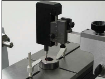
Checking of small plain ring gages from Ø 2 mm as standard
