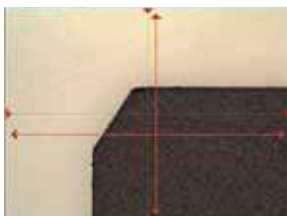
(1) The next measuring point is indicated with red cross hairs.
