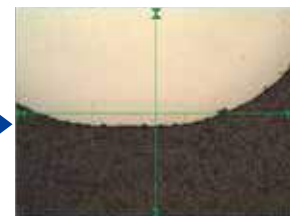
(3) When both cross hairs overlap one another while indicating the target point, press the Input button to complete the measurement.
