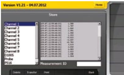
Window that allows you to view, transfer and print the recorded values for each channel
