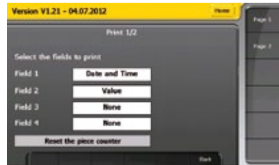
Select the information that will be printed when it is sent by pressing the pedal or external contacts
